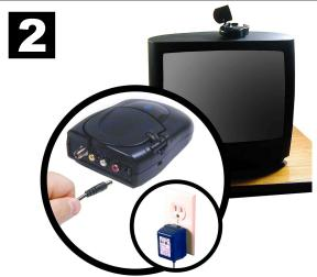
Connect the wireless video receiver to power and plug it into a wall outlet.
